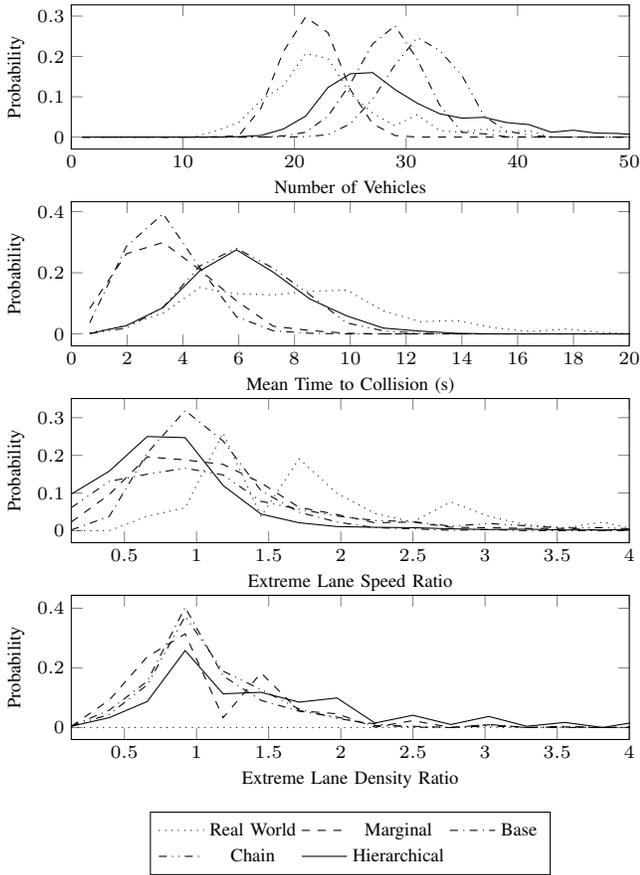
Fig. 5: Distributions over metrics from sampled scenes from Highway 101 section 101b. The extreme lane density ratio for real-world data approaches infinity due to the lack of vehicles in the auxiliary lane.
