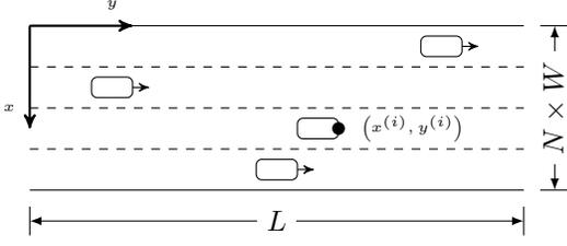
Fig. 1: Lane-relative frame for a straight multi-lane highway
